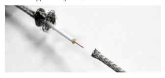
**4.** Repeat steps 1-3 on other side of splice. You should now have room for the solder splice connector.
