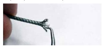
**3.** Push braid back until ½" of inner wire is exposed. Use wire strippers to expose 3/16" of inner conductor.
