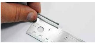
2. Separate the end fibers of the stainless steel braid.
