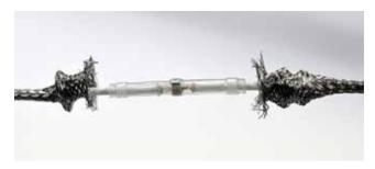
**6.** Use a hot air gun or butane flame to shrink the splice and solder the wires. Hold the splice steady while the solder is liquid to ensure a good connection.
