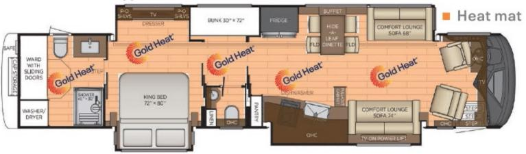
Underneath a coach's tile floor lies custom-made, radiant-floor heat mats specifically designed for the mobility and power needs of a luxury motorcoach. These heat mats run on electricity - approximately 15W per square foot.
