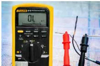
Figure 2. Confirm no continuity to ground wire.
